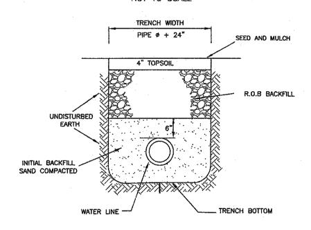
BACKFILL SHALL BE RUN-OF-BANK GRAVEL COMPACTED IN 6" LIFTS.
