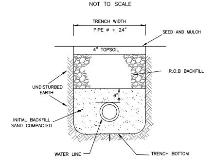
BACKFILL SHALL BE RUN-OF-BANK GRAVEL COMPACTED IN 6" LIFTS.
