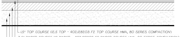
L 2.5" BINDER COURSE (19 BINDER - 402.198902 F9 BINDER COURSE HMA, 80 SERIES COMPACTION) L 3.5" BASE COURSE (37.5 BASE - 402.378902 F9 BASE COURSE HMA, 80 SERIES COMPACTION) L 12" GRAVEL SUBBASE (NYSDOT 733-04 SUBBASE COURSE, TYPE 2) - APPROVED GEOTEXTILE (SEE NOTE)
