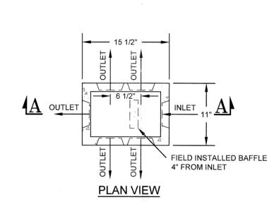
PROVIDE WATERTIGHT JOINTS AT ALL INLET/OUTLET PIPES OUTLET TO NEXT DROP DISTRIBUTION BOX TO CONCRETE SLOPE 1"/FT ALONG COVER \ PER ASTM 2729 PIPE RUN . 4" SOLID PVC PER ASTM 2729 12" MIN SAND OR PEA GRAVEL
