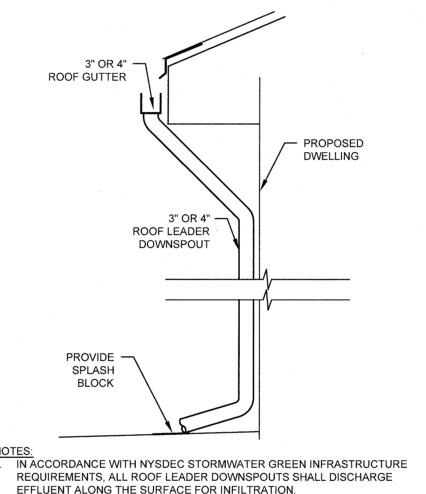
EFFLUENT ALONG THE SURFACE FOR INFILTRATION. 2. CONNECTION OF ROOF LEADERS TO CLOSED SYSTEMS IS PROHIBITED. HOMEOWNERS SHALL MAINTAIN SPLASH BLOCK LAWN AREA AS SHOWN ON THE PLANS TO PROVIDE INFILTRATION OF STORMWATER ROOF RUNOFF.
