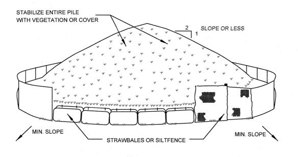
NOTES: 1. AREA CHOSEN FOR STOCKPILING OPERATIONS SHALL BE DRY AND STABLE. 2. MAXIMUM SLOPE OF STOCKPILE SHALL BE 1:2. UPON COMPLETION OF SOIL STOCKPILING, EACH PILE SHALL BE SURROUNDED A WITH EITHER SILT FENCING OR STRAWBALES, THEN STABILIZED WITH VEGETATION OR
