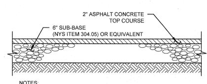
ITEM NUMBERS REFER TO NYSDOT SPECS. PAVEMENT TO EXTEND FROM CURB TO RIGHT OF WAY LINE. DRIVEWAY PAVEMENT SECTION
