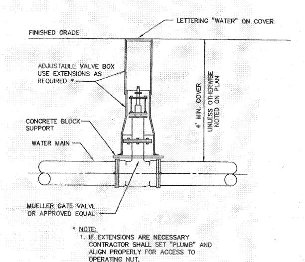
VALVES-RESILIANT SEAT (AWWA-C509) TYPICAL GATE VALVE DETAIL NOT TO SCALE
