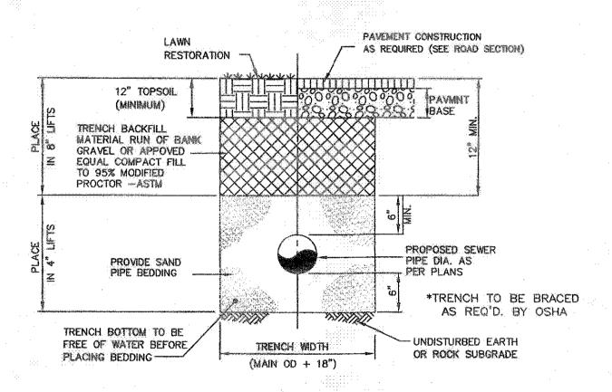
TYPICAL SEWER TRENCH DETAIL NOT TO SCALE
