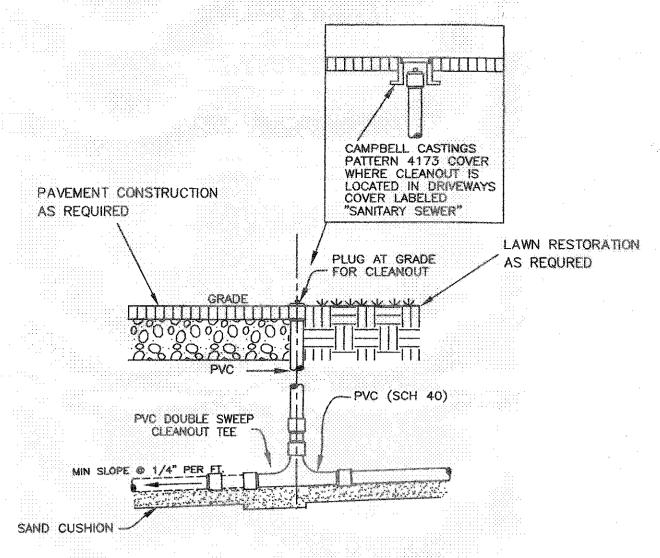
SEWER LATERAL CLEANOUT DETAIL NOT TO SCALE
