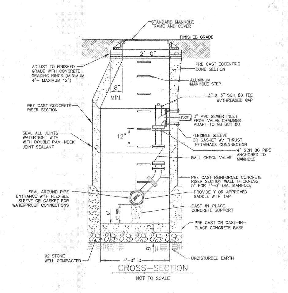
SEWER MANHOLE W/ FORCE MAIN CONNECTION DETAIL NOT TO SCALE
