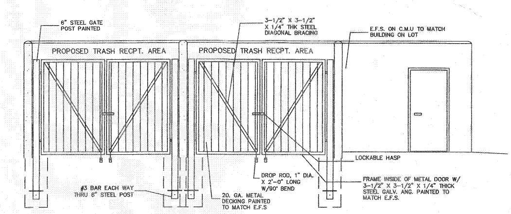
DUMPSTER RECEPTACLE SCREEN ELEVATION SCALE: NOT TO SCALE
