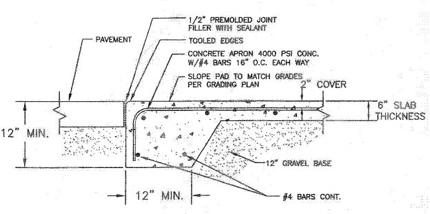
DUMPSTER CONCRETE PAD DETAIL NOT TO SCALE
