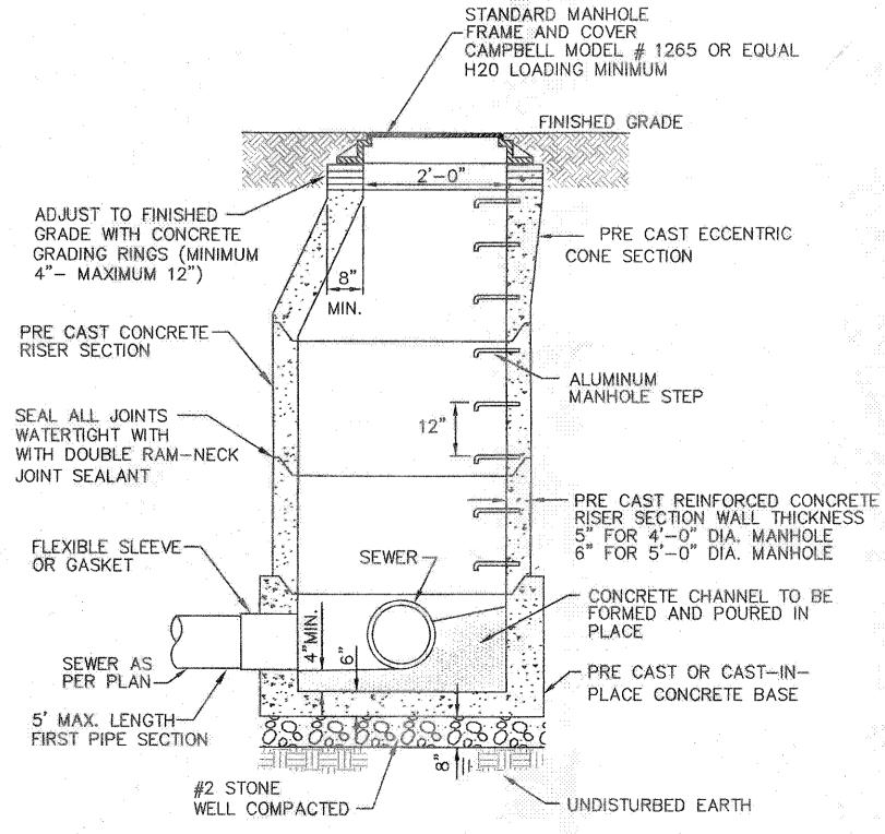
TYPICAL SANITARY SEWER MANHOLE NOT TO SCALE
