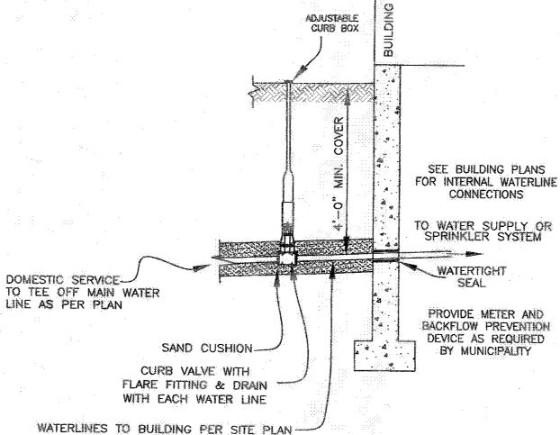
TYPICAL WATER LINE CONNECTION NOT TO SCALE
