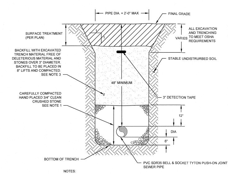
1. ALL FILL BELOW BUILDING AND PAVEMENT TO BE COMPACTED TO 95% MAXIMUM DRY DENSITY AS DETERMINED BY MODIFIED PROCTOR TEST.
