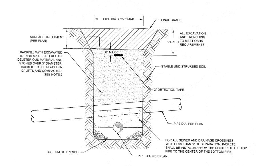
SEWER & DRAINAGE CROSSING WITH LESS THAN 6" SEPARATION BETWEEN PIPES
