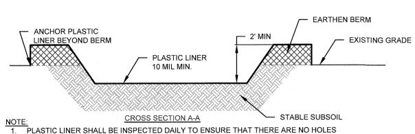
CLEANING OF THE WASHOUT FACILITY. WASHOUT FACILITY SHALL BE LOCATED A MINIMUM OF 100 FEET FROM DRAINAGE SWALES, STORM DRAIN INLETS, WETLANDS, STREAMS OR OTHER SURFACE WATERS.
