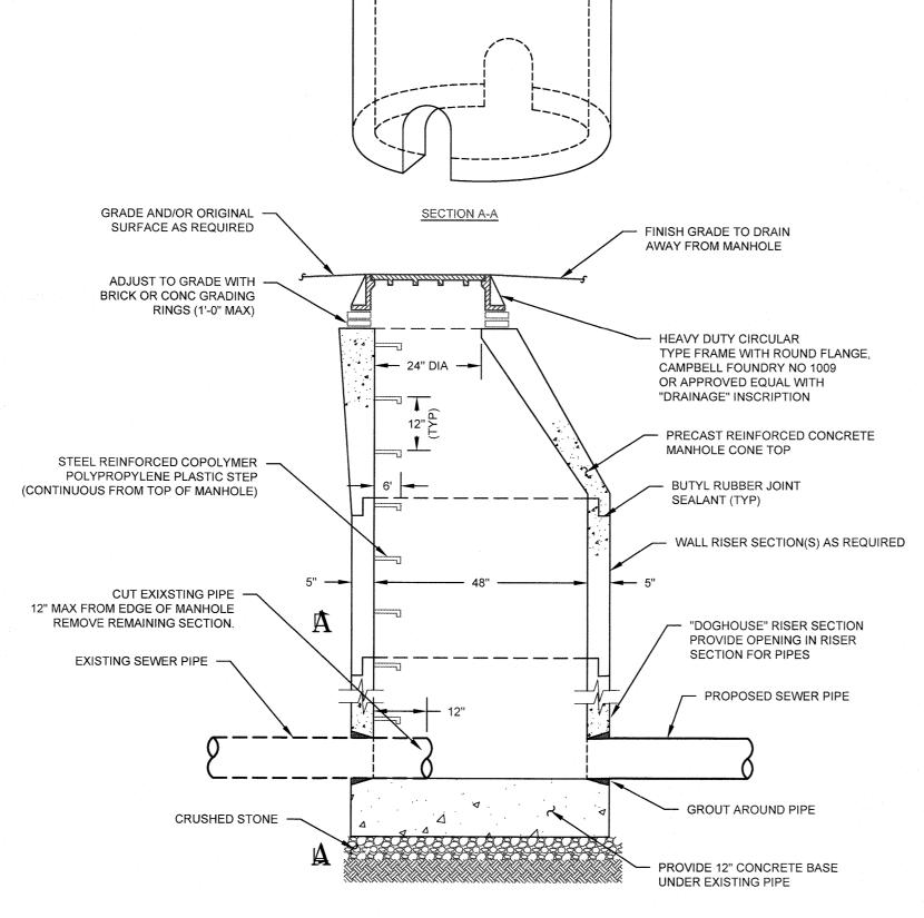
CONCRETE TO HAVE A MINIMUM COMPRESSIVE STRENGTH OF 4000 PSI AT 28 DAYS. REINFORCEMENT TO BE IN CONFORMANCE WITH ASTM A615GRADE 60 AND ASTM
