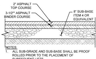
SUBSEQUENT LIFTS. 2. MATERIAL THICKNESS SPECIFIED IS "AFTER"
