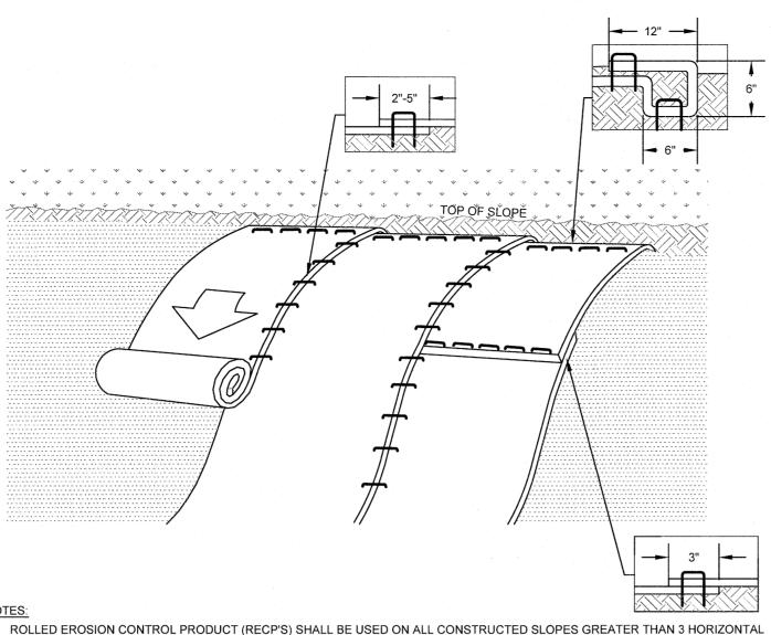
1. ROLLED EROSION CONTROL PRODUCT (RECP'S) SHALL BE USED ON ALL CONSTRUCTED SLOPES GREATER THAN 3 HORIZONTAL
